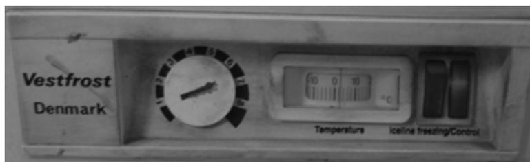
**Figure 9.8.** The temperature reader of an ILR
