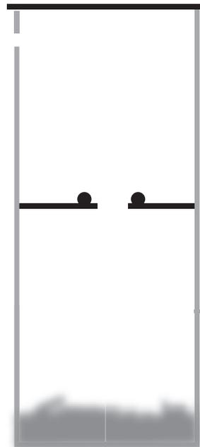
Figure 5.15. A bore hole latrine<sup>226</sup>
