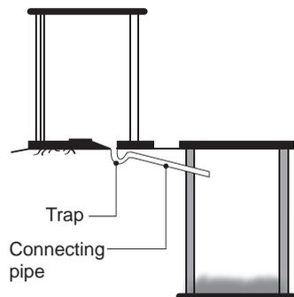
Figure 5.18. Water seal latrine<sup>228</sup>
