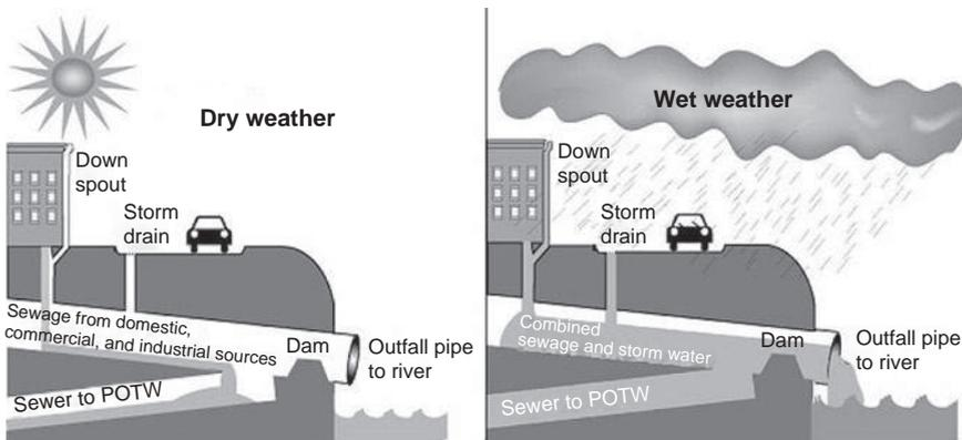
Figure 5.21. Combined sewer overflow
